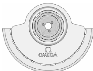
Rotor with ball bearing and spring clip Ref. XXXX/1026
