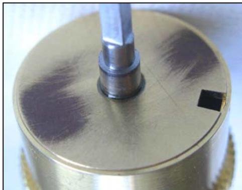
Visible ring of oil around barrel arbor
