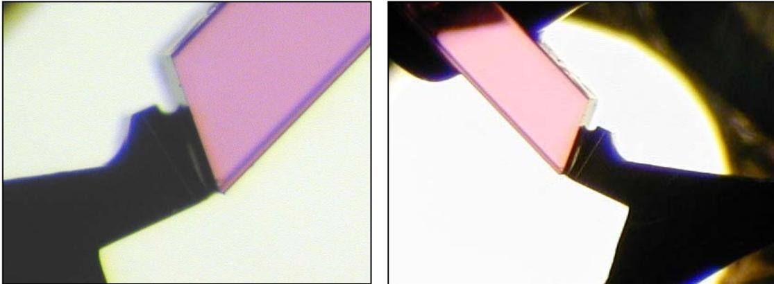
The correct amount of oil is visible on the impulse face, a trace of oil can be seen on the locking face but no oil should be present on the other surfaces of the pallet jewels.
